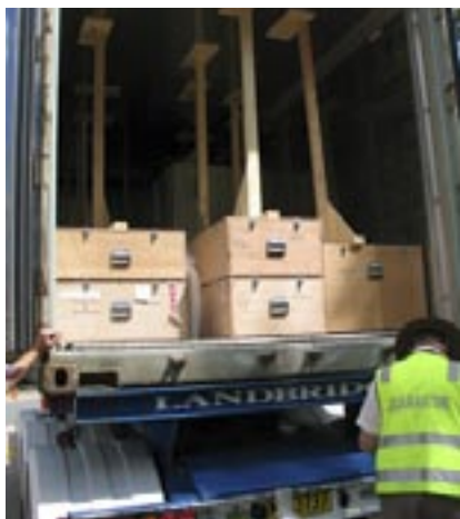
REEFER CONTAINERS ARE RECOMMENDED FOR THEIR AIRTIGHT SEAL AND ABILITY TO MAINTAIN A CONSTANT TEMPERATURE.
