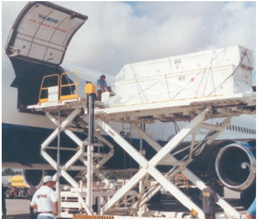
LOADED PALLETS AND CONTAINERS ARE WEIGHED BECAUSE A PLANE MUST BE LOADED IN A SEQUENCE WHICH MAINTAINS IT'S BALANCE IN FLIGHT.
