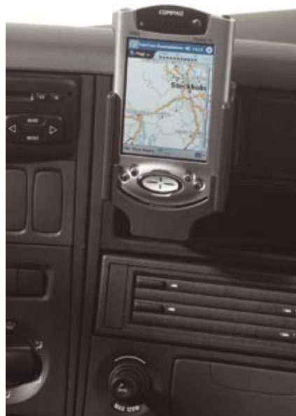
A GPS RECEIVER AND A MOBILE PHONE SIT SIDE-BY-SIDE AND AT REGULAR INTERVALS THE PHONE SENDS A TEXT MESSAGE VIA SMS CONTAINING THE DATA FOR THE GPS RECEIVER TO ANALYSE.
